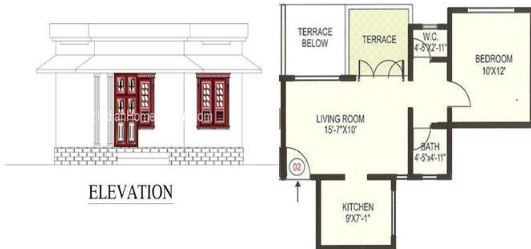
Figure1. Elevation and Plan of Residential Building
